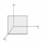
b) Imagine a charge q at the center of a cube of edge length 2L. Then:  $\Phi = q/\varepsilon_0$ . Here the square is one 24th of the surface area of the imaginary cube, so it intercepts 1/24 of the flux. That is,  $\Phi = q/24\varepsilon_0$ .
